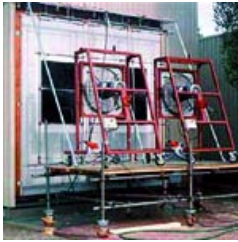
Figure 5.58 Testing of air and water tightness in a laboratory
