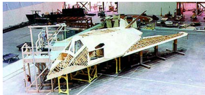
Figuur 5.44 Houten mockup van de Lockheed F117 Stealth Fighter
