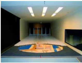
Figure 5.54 Windtunnel research of an urban situation
